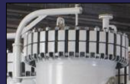
Quick closure with swivel bolts, detail.
