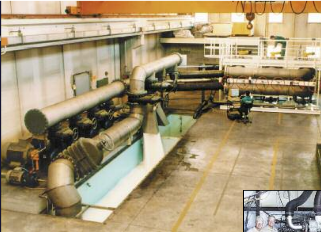
Water test rig, 4,200 m 3 /h (18,500 GPM)
