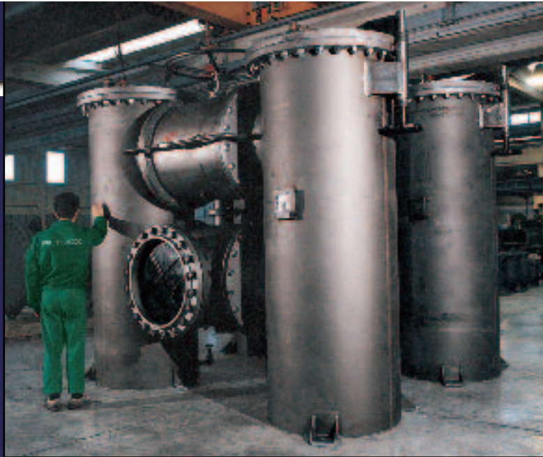
DX filter with change-over pressure-seal valve.
