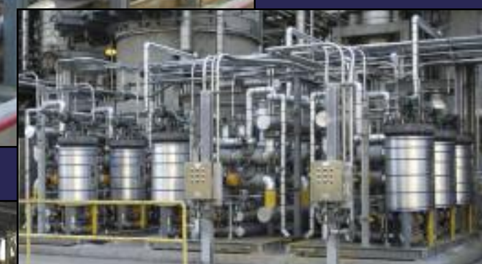
ACR feed filter for Hydrocracker Unit (Blend of HCGO/HVGO) Port Arthur, USA
