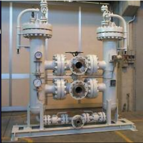
DX filter with change-over pressure-seal valve.
