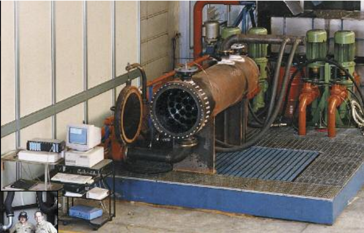
Test rig for lube oil and heavy fuel oil, 300 m 3 /h (1,320 GPM).
