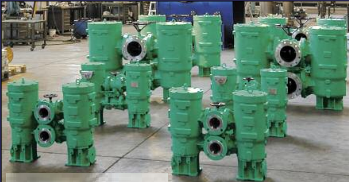
DX filter with change-over pressure-seal valve.
