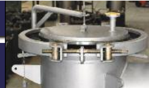
C-clamp quick closure, detail.
