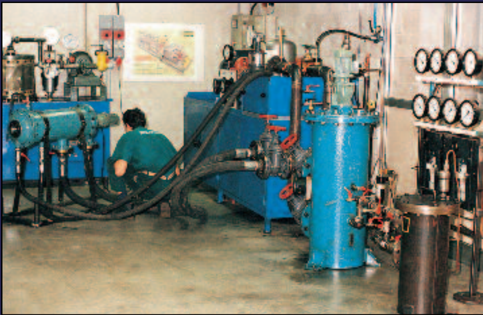
Test rig for heavy fuel oil 30 m 3 /h (132 GPM).
