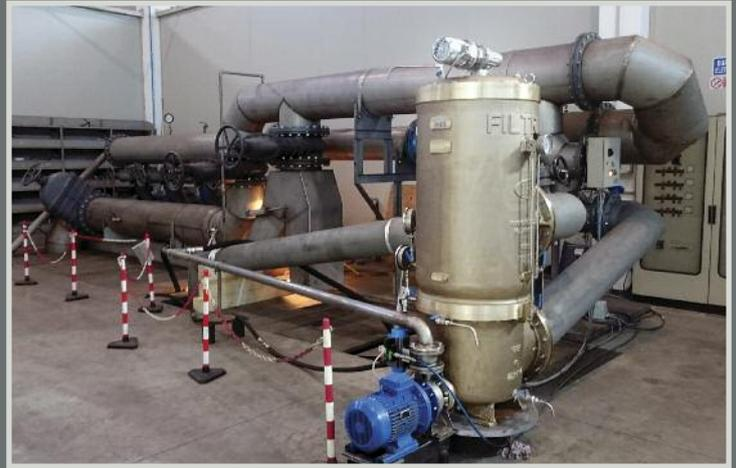
Filter ACB-9100 on test bench: Flowrates up to 4.200 m<sup>3</sup>/h
